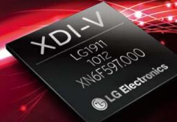
XDI-V ISP Technology is engineered to process high quality images from 520K/610K sensors so as to guarantee 650 TV Lines(color) / 700 TV Lines(B/W). Also, the package size is 46% smaller than the existing one, and the high technology process and low power consumption design reduce power consumption by 20~30%. The newly improved 2D+3D-DNR reduces noise and after-images, enabling an optimal monitoring even at low light. Now experience XDI-V that supports Multi languages and coaxial Communication.
