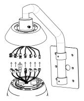
5. Assemble the camera to the mounting adaptor by turning it clockwise. Tighten the M3 SAMS Screws and then align the cover adaptor and main body.
