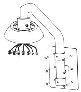
3. Connect the safety cable to the camera. 4. Connect the cables to the camera jack.
