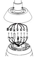
3. Connect the safety cable to the camera.
