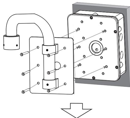
Use the supplied wrench to tighten the screws.
