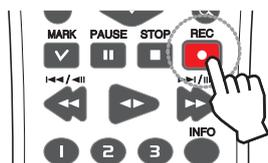
2. Press the REC button and then press the channel button you want to stop recording. If you stop instant recording, the recording mode will be changed into the scheduled recording mode (Continuous/ Sensor / Motion records). If the schedule is not set, the button indicator turns off and the recording type indicator turns gray on the selected channel screen of the main monitor.
